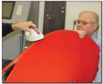
Fig. 8: Applying fabric to a curved perimeter is best done with two people. Bill Griffin holds the panel in place while the author pulls and irons the fabric.
