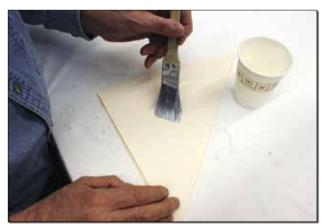
Fig. 2: In addition to the parts being covered, Oratex adhesive must also be applied to the backside of the fabric.
