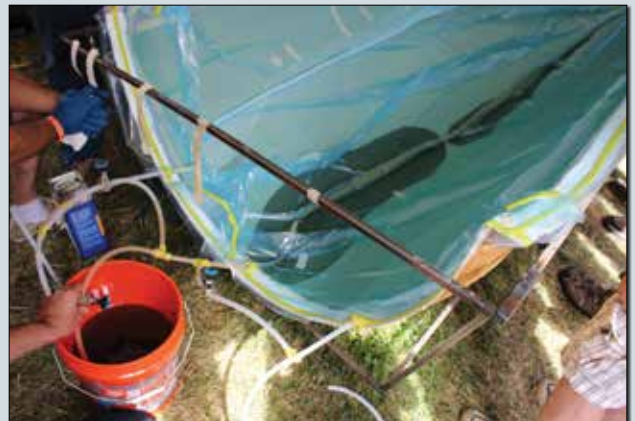
And we're off! The center inlet hose is submerged in the resin bucket, the valve is opened, and atmospheric pressure forces resin into the mold.
