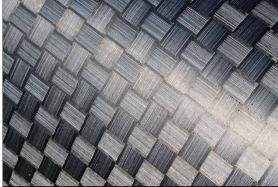
Fast forward 12 hours. Here's the surface of the laminate after removal from the mold. Note lack of voids and bubbles. Black fibers are carbon, white fibers are Innegra olefin.
