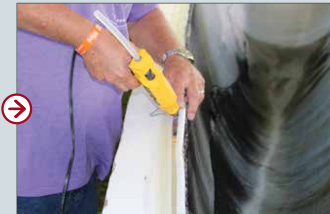
Hot glue gun is used to attach MTI (Membrane Tube Infusion) vacuum hose to the perimeter of the mold. It only needs a dab here and there, just enough to keep it in position until...
