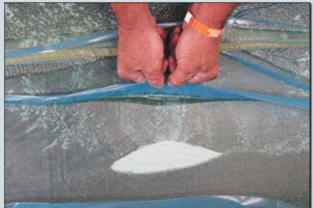
There were a few dry spots, but these guys had a trick. Just pull and release a fold in the bagging film to "pump" resin into the dry area. Experienced operators may also use a vacuum needle (a small probe connected to the pump tubing), which can be poked through the bag to focus vacuum on a dry spot. As the probe is withdrawn, the hole is sealed with a bit of tacky tape.
