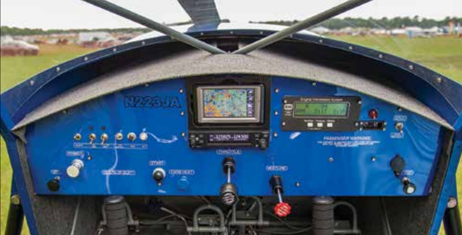
The KIS principle at work; GPS, radio, engine monitor, and an ELT head.
