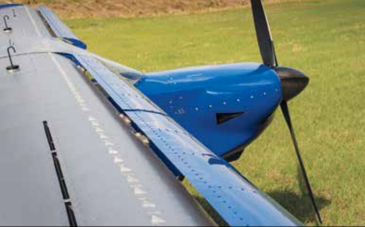
Leading edge slats extend automatically.
