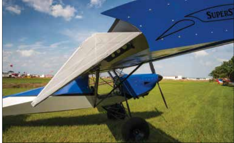
The ailerons can now be teamed with a spoiler system.
