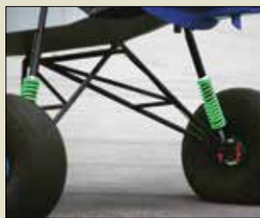
Prototype coil-over "test mule" struts for the SuperSTOL.
