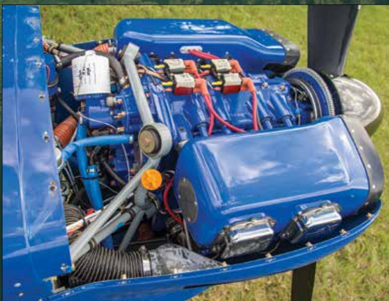
Titan 340 with prototype twin plenums and Lightspeed ignition.
