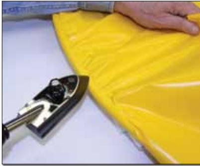
Fig. 7: With enough effort and heat, the fabric can be wrapped around compound shapes without puckering.
