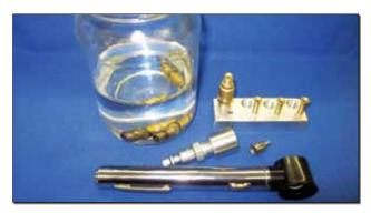
Gun cleaning solvents are popular for soaking injectors, but be aware that some of them can etch brass. Carburetor cleaner spray from the auto parts store is mostly toluene, acetone, and MEK; any or all of them can be used to soak injectors. The best approach is an ultrasonic cleaning vat.
