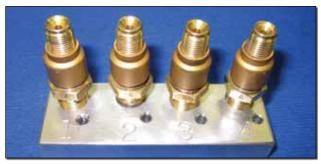
back in the wrong cylinders, nor do you want to swap nozzle inserts between injector bodies. The tool is just a small block of aluminum scrap tapped 1/8 inch NPT for the bodies, drilled for the inserts, and marked with cylinder numbers.
