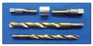
The first simple tool is a threaded bushing. One end is tapped for an air chuck fitting. The other is tapped 1/8 inch NPT to match the male thread on the injector body. Screw the injector into the tool, chuck the tool to an air line, and the injector is blown out with the full air line volume.
