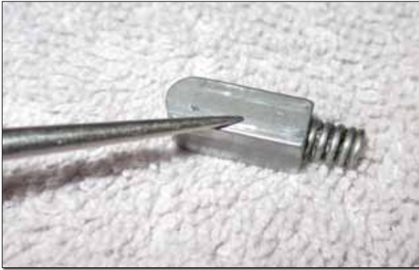
Inspect the square pin. Burrs, scars and gouges are common.
