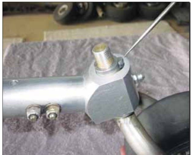
Let's reassemble. Clean and grease the main bore. Grease the pin and its recess. Slide the pin and spring into the recess, push in the pin until flush with the shaft surface, and slide the shaft up into the main bore. If the fork points rearward, the pin will snap into the slot when the shaft is fully inserted. The fork assembly will not fall out.
