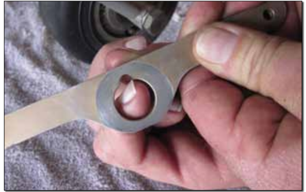
Last, clean the control arm and inspect carefully right at the ends of the half-moon cutout. If burred, use a file or stone, but do not round off the sharp corner. If the corner is worn to a rounded shape, your best bet is a new arm.
