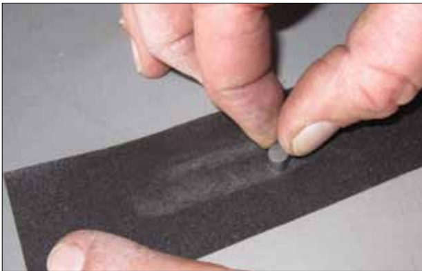
Lay a new sheet of 400 or higher grit on a hard, smooth surface. Lap the pin surfaces until the bumps and burrs are gone. Clean it carefully.
