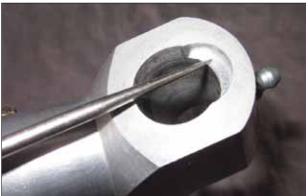
Inspect the slot adjacent to the main bore. Again, smooth and clean are the operative words.
