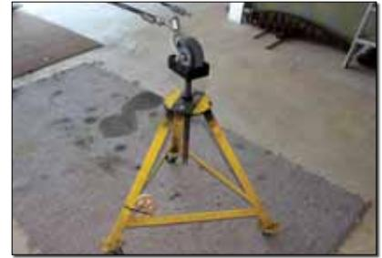
Fig. 4: Engine stand converted into a tailwheel stand.
