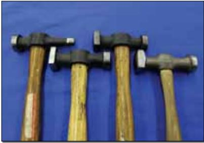
Fig. 2: Modified cast copies of high-quality forged hammer (on right).
