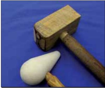
Fig. 9: Shop-made wooden mallet and fancy nylon hammer.
