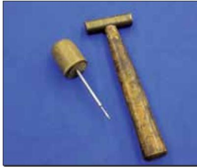
Fig. 10: Brass hammer and tool to push blind rivets into holes.
