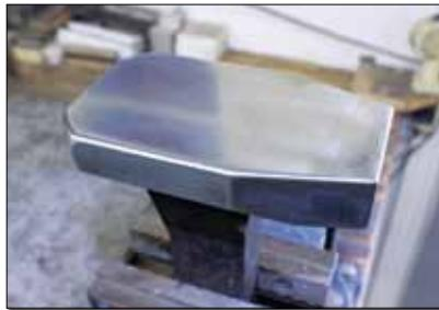
Fig. 5: Scrap steel used like an anvil for metal forming.
