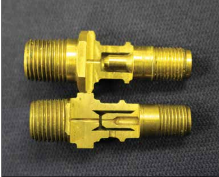
Figure 10: Injector nozzles. (Top) Current two-piece nozzle with swappable restrictor insert. (Bottom) Older Bendix nozzle with pressed insert. Note air bleed passage through the side wall of the nozzle body at the bottom of the photo.
