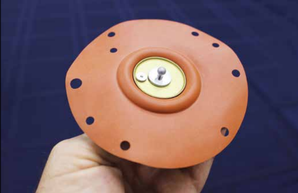
Figure 6: Control body fuel diaphragm with bleed fitting and ball valve.
