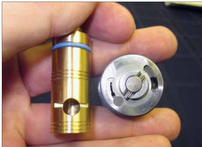
Figure 5: Airflow Performance mixture valves, early drum type on left, later disk valve on right.
