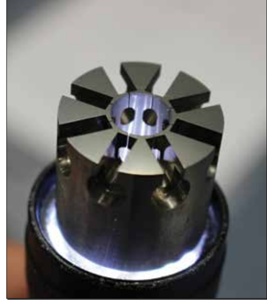
Figure 8: Flow divider insert showing metering slots and unrestricted outlet holes in valve piston passage.
