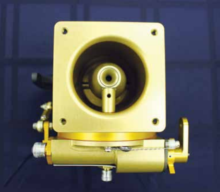
Figure 3: AFP FM-150 showing straight throat and mast-mounted high gain venturi.
