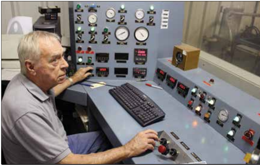
Monty Barrett at the console. Engine control on the operator's right, water brake and air controls on the left. Monty is scanning a bank of engine instruments, here off camera.
