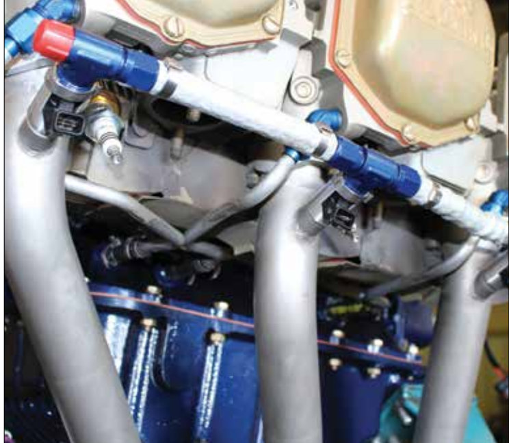
Left side fuel rail assembly. Individual Siemens injectors squirt into the Lycoming intake pipes via welded ports. Hoses link injectors so they all share a common supply at a fixed pressure.
