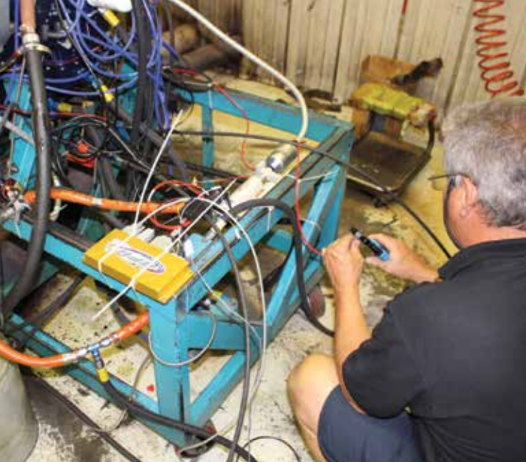
Robert Paisley wiring and plumbing EFii components. SDS ECU (gold box) and fuel pump module are simply strapped to the dyno frame. Looks messy, but it's strictly temporary.
