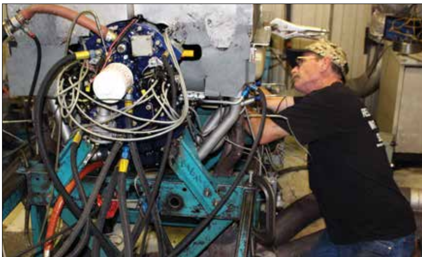
Allen Barrett makes an adjustment. The big silver box over the engine is an air hood. A 25-hp electric fan ensures enough cooling air supply.
