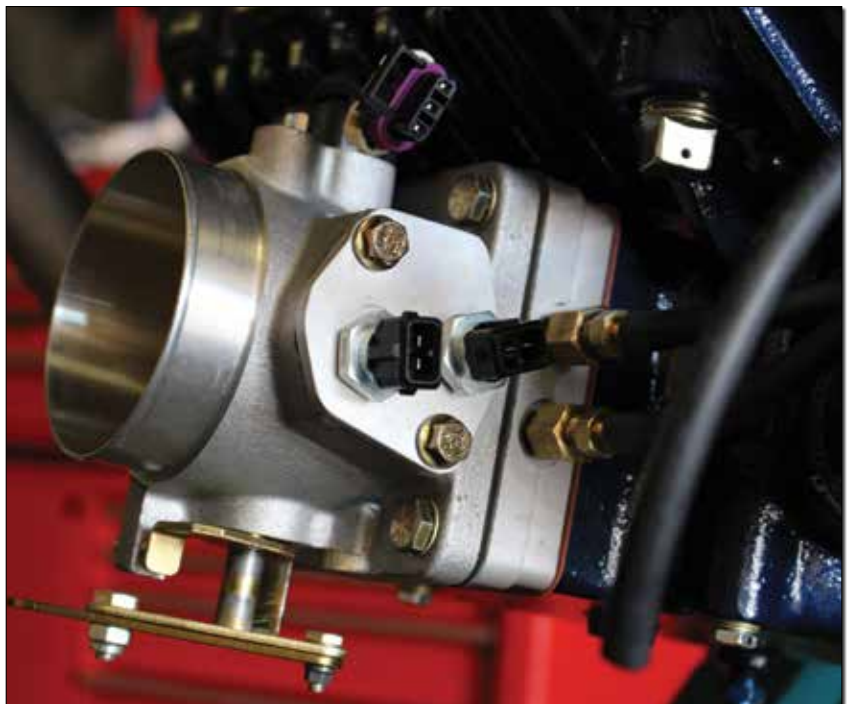
The EFii system uses a slightly modified 80mm BBK-brand throttle body for air control. The air temperature sensor connectors (two for a dual ECU system) are facing the camera. The throttle position sensor is on top. No mixture control; that's electronic.
