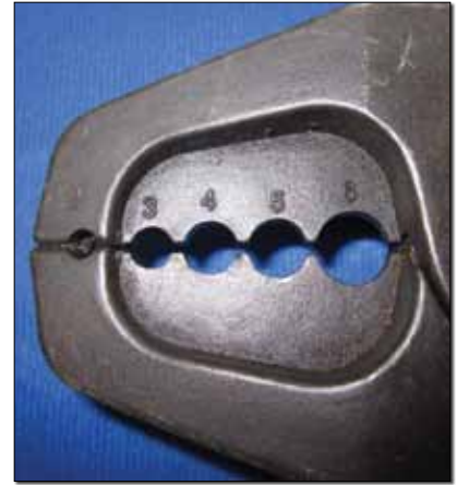
Fig. 14. For oval swage sleeves, the numbers on the Continental/GBG S-2236H jaws correspond to multiples of 1/32 inch. The same is not true for stop sleeves.
