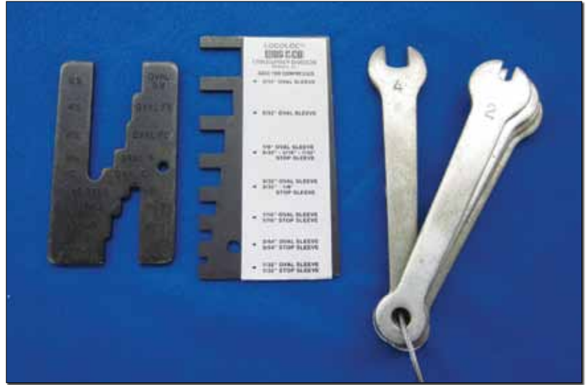
Fig. 18. We found minor variations between gauges from (left to right) Nicopress, Locoloc, and Continental/GBG.
