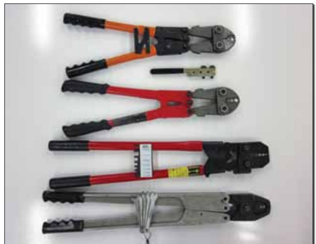
Fig. 16. Available crimp tools include (from top) Nicopress CGMP, inexpensive bar-type, cheap Nicopress knockoff, Locoloc 1-SC, and Continental/GBG S-2236H.
