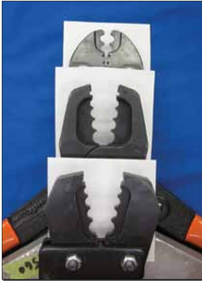
Fig. 17. Jaw openings of (from top) Nicopress CGMP, Continental/GBG S-2236H, and Locoloc 1-SC.
