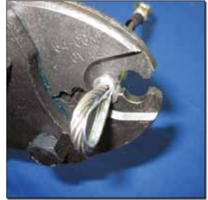
Fig. 9. Position the sleeve in the correct groove of the tool and squeeze.
