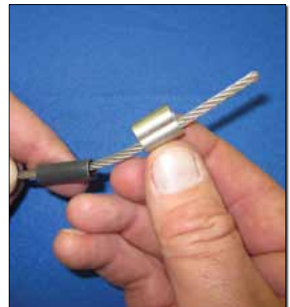
Fig. 6. Slip the cable through a short length of adhesive heat shrink, then the sleeve.
