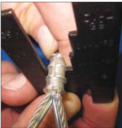
Fig. 10. Use a gauge on every crimp, measuring what was formerly the widest part of the sleeve.
