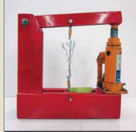
Fig. A. To examine performance at various crimp dimensions, multiple cable assemblies were crimped and pulled to destruction.
