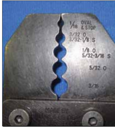
Fig. 13. Three of the grooves in the Locoloc 1-SC are marked with multiple fractional sizes. Note the “O” and “S”, which mean “oval sleeve” and “stop sleeve”.
