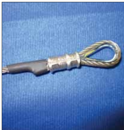
Fig. 11. Slide the previously installed heat shrink tube over the tail and warm it with a heat gun.
