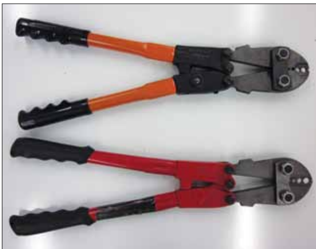
Fig. 15. A Nicopress 64-CGMP (top) and a $30 knockoff (bottom) may look the same, but the copy didn’t include a gauge and didn’t crimp to the correct dimension.
